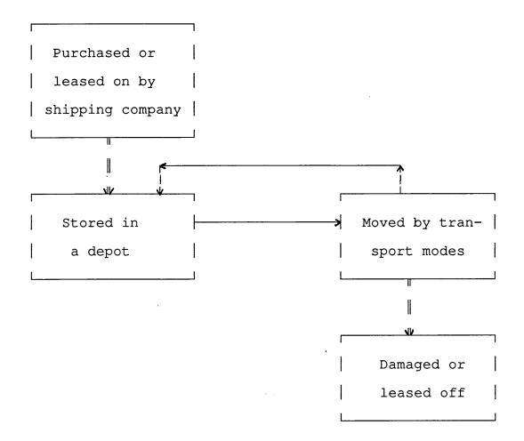
The above figure illustrates that a container shipping company purchases, or leases on, a container as long as there is new cargo demand for that extra container. It then stores it in company's depot or other warehouse designated by company for subsequent cargo use. Movement of the container includes
